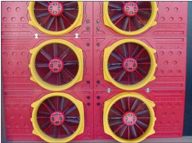
Conducting whole building performance for air tightness. Photo courtesy of Retrotec www.retrotec.com
